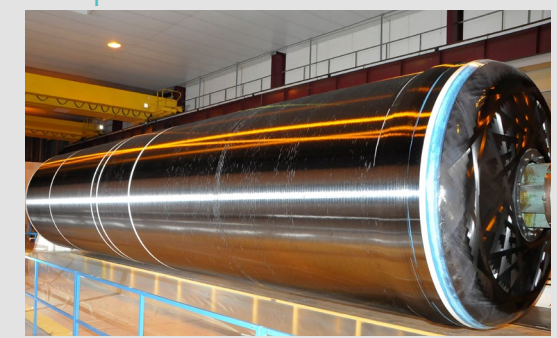
Filament wound structure with polyurethane internal elements
