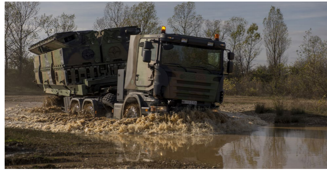
The 6x6 prime mover with semi-trailer offers high land mobility on rough terrain
