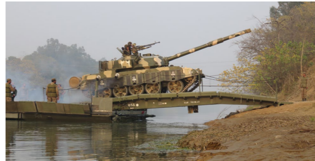
Multi purpose tactical ramp* : / no bank preparation / interoperability with other floating bridges / dry gap crossing
