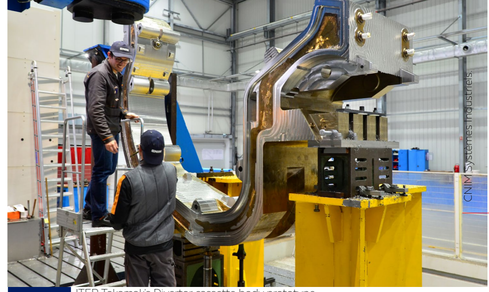
ITER Tokamak's Divertor cassette body prototype 3.3x2.5x0.8 m – 316LN & XM-19
