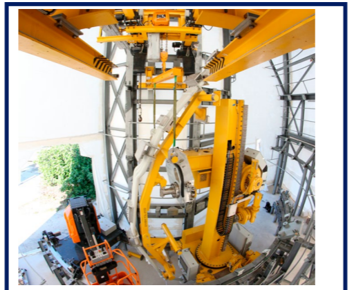
IN-VESSEL TOWER CRANE (IVTC) - ITER / Handling equipment used for the initial assembly in vessel components / Confined working space / Millimetre accuracy achieved
