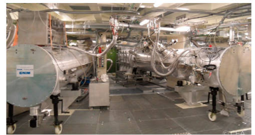
Diagnostic insertion system for inserting various types of plasma diagnostics in the Megajoule Laser project. The remotely-controlled diagnostic insertion systems operate under vacuum conditions
