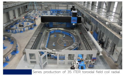
Series production of 35 ITER toroidal field coil radial plates using electron beam welding under local vacuum.
