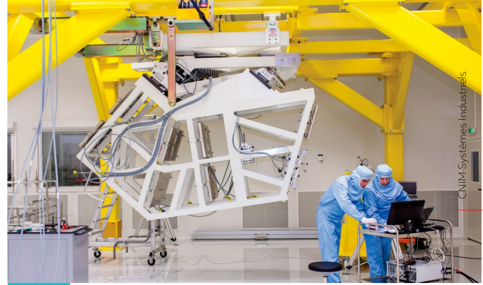
Handling system for the Megajoule Laser Frequency and Focusing Conversion System for positioning mirrors to within a few \mu\text{m} ; ISO7 compatible and capable of bearing loads of several tonnes.
