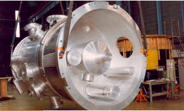
Electron beam welding of the vacuum chamber of the Heinz Maier-Leibnitz (FRM II) research reactor's neutron source
