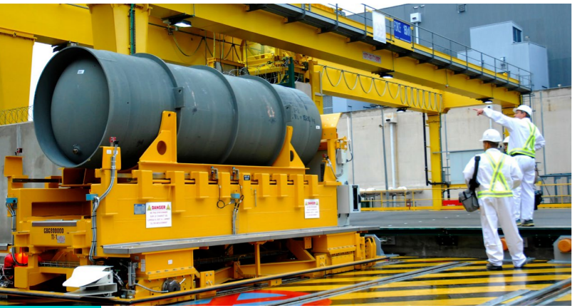
Enriched uranium handling system (GBII plant)
