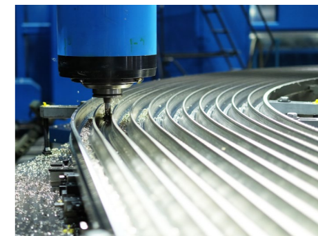
Serial production of 35 radial plates for ITER
