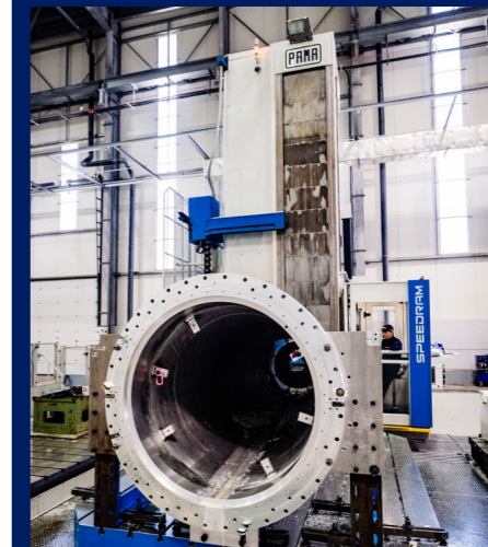
Machining of under pressure nuclear equipment for Laue-Langevin Institute
