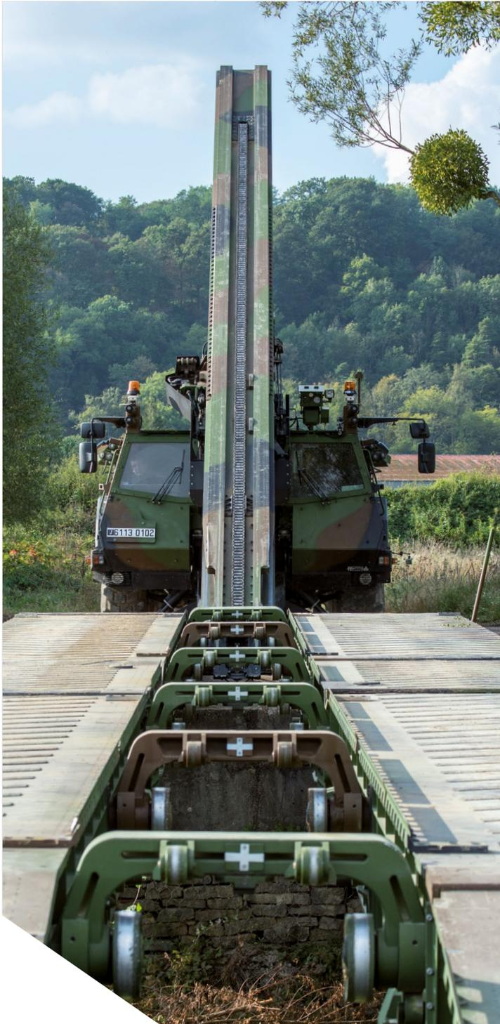
In combat conditions, the PTA offers a high capability crossing to support heavy & medium mechanized Forces.
