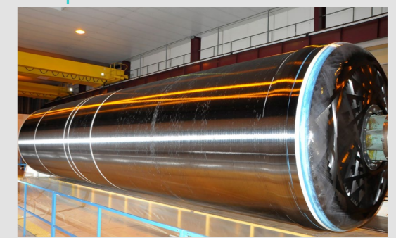
Filament wound structure with polyurethane internal elements
