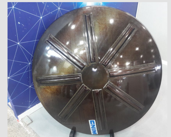
Reinforced composite: Liquid Resin Infusion (LRI) technique for aircraft radome (Forward Pressure Bulkhead)
