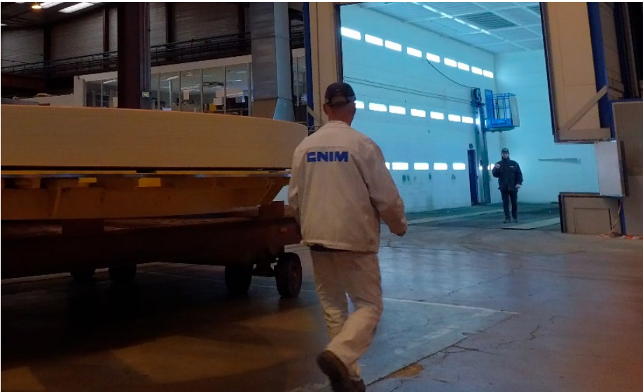
Large ovens: up to 3,5 x 3,6 x 16 m³ of useful volume.
