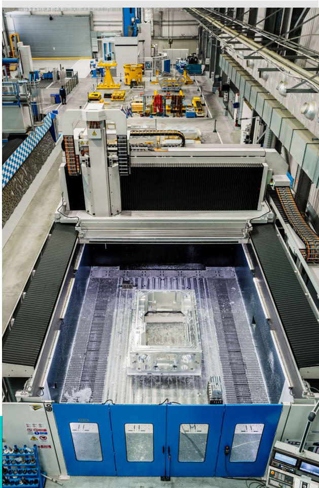
Double gantryl milling machine (X 30000, Y 9000, Z 1250 mm, maximum load: 5 tons / sqm).
