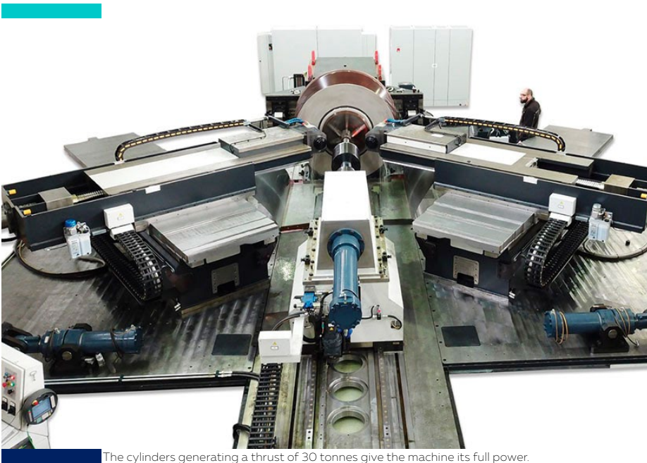
The cylinders generating a thrust of 30 tonnes give the machine its full power.
