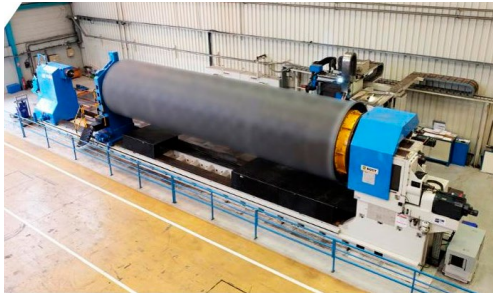
Horizontal lathe (L 15000 mm, maximum load 40 tons).
