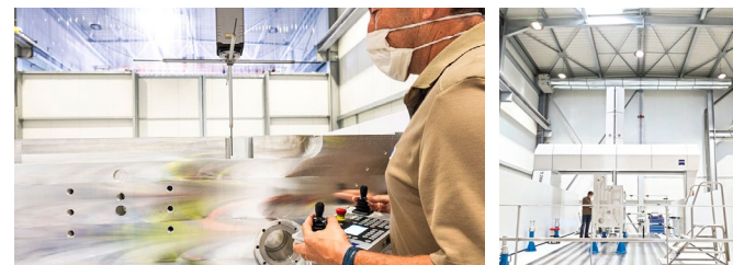
Control to the nearest 1/10 th of a millimetre with the ZEISS MMZ-G machine: X4,000 X Y8,000 X Z2,000 mm
