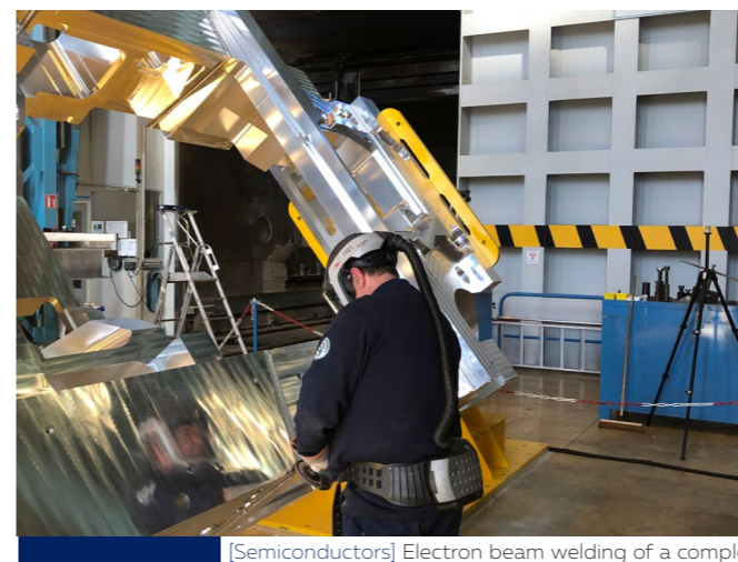
[Semiconductors] Electron beam welding of a complex geometry and large machine frame.
