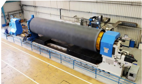
Tour horizontal (L 15000 mm, charge max. 40 tonnes).
