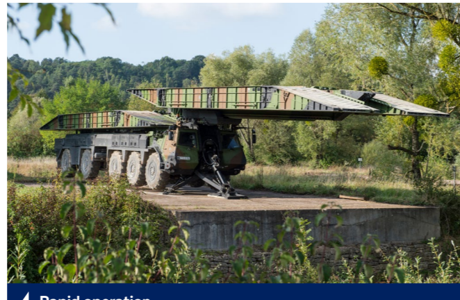
▲ Rapid operation Short bridge (14 m) in 8 min / Long bridge (26 m) in 10 min
