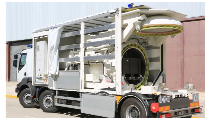
▲ Tank strength: 13 kg eq. TNT
